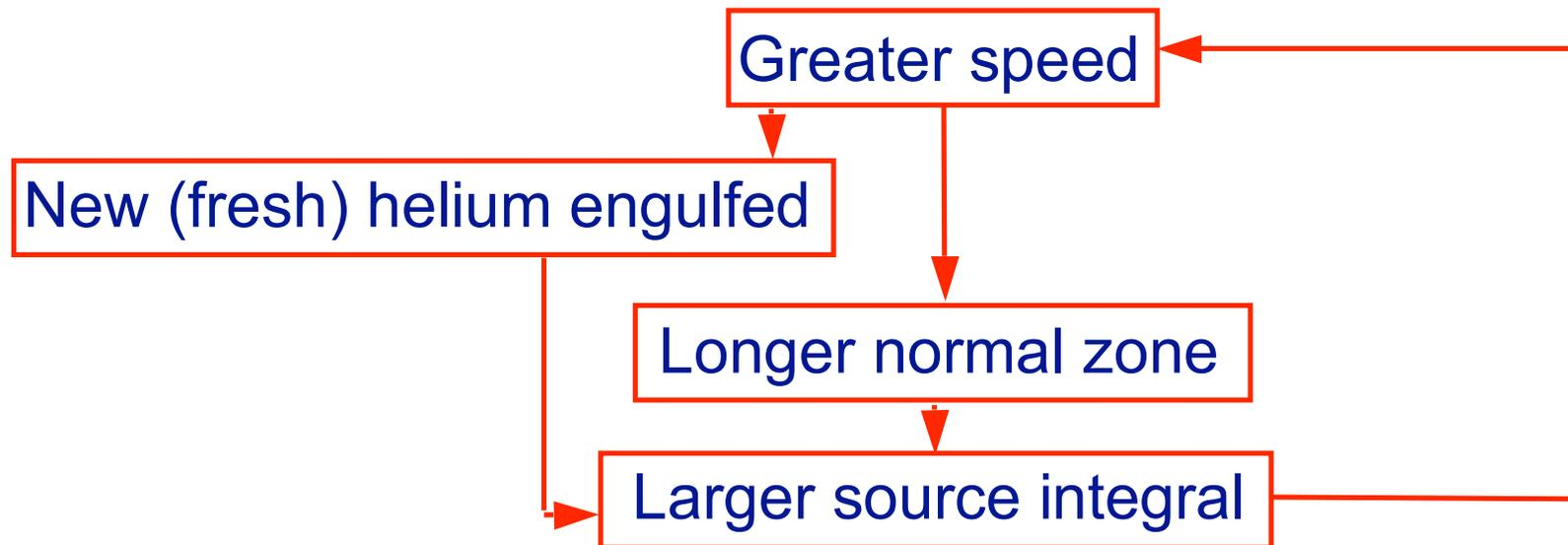
☞ Quench propagation at increasing speed
