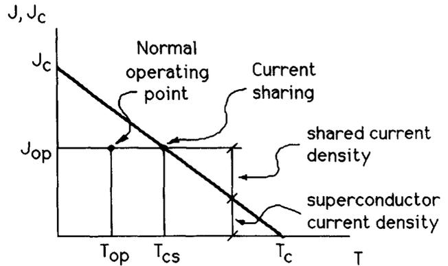
Figure 2 Operating point and definition of the current sharing temperature in the case of linear  $J_c$  versus  $T$  dependence. The effect of the increase of the operating temperature is also indicated by the shared current density
