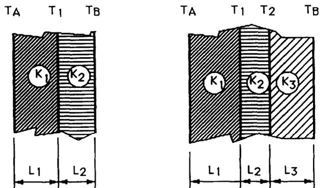
Figure 10 Configurations considered for the calculations of the thermal resistance of the links. The values of the temperature at the boundaries of the slab are given
