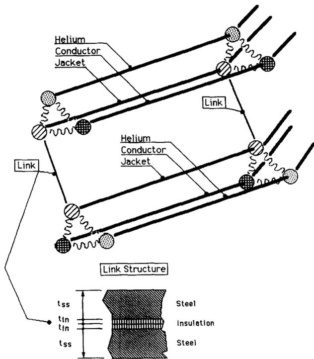
Figure 9 Schematic view of the details of the coupled 1-D channels equivalent to the initial 3-D problem. The internal structure of the coupling links is shown
