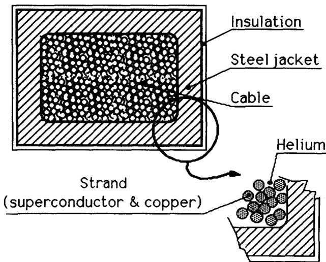
Figure 3 Schematic view of the cross-section of the conductor configuration assumed
