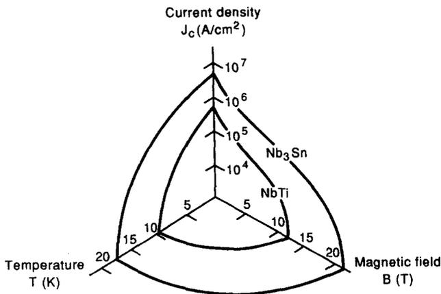
Figure 1  $J_c(B, T)$  surfaces for Nb<sub>3</sub>Sn and NbTi
