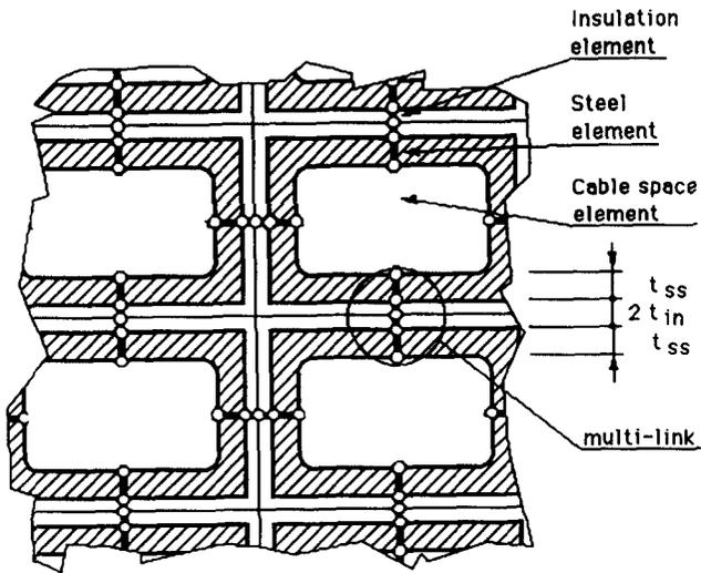
**Figure 7** Equivalent multi-link model for the heat flux in the winding pack. The sandwich of jacket and insulation is substituted by a series of thermal resistances with degrees of freedom lumped at the centre of each layer of the sandwich
