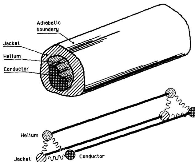
**Figure 6** Schematic view of the 1-D model used for the conductor in the longitudinal direction
